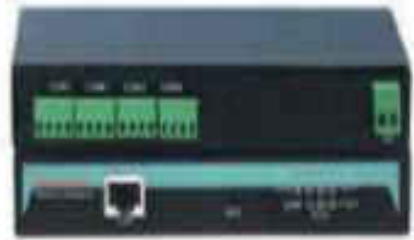
Ethernet-Modbus Gateway to 4-Port RS-485/422
